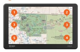
The Main page displays the current map, with your position shown by an indicator in the centre of the screen. Functions include:
